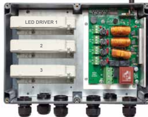
4-Channel Controller with optional LED drivers installed
